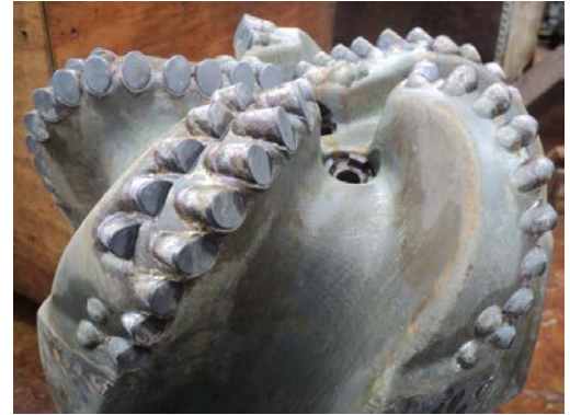
Dull grade of 1-1-WT-A-X-I-NO-TD achieved for this field record ROP and footage run.
