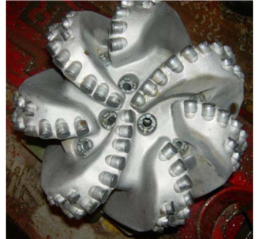
Photo of Dull Bit with Rig Grade of 1,3,WT,S,X,O,HC,PR
