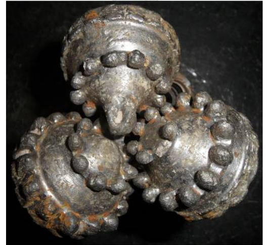
This is the typical appearance of a milltooth bit after drilling through frac plugs. The inner rows remain in good condition while the outer rows are worn beyond recognition due to the hard outer slips.
