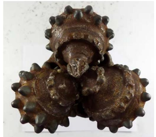
After drilling 59 composite plugs, this SRP received a 4-1-WT dull grade.
