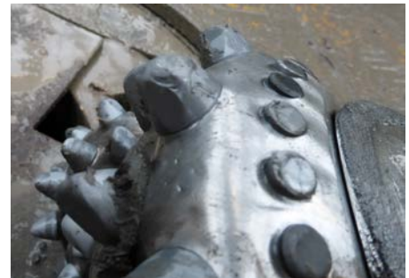
This bit also features Varel's diamond capped TCIs in strategic locations along the back row to provide added protection.
