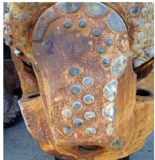
Receiving a 1-1-WT-A-E-IN-NO-TD dull grade, this A-Force design complete with EdgeGuard technology withstood 1,301 ft of the Berea and Ohio formations.
