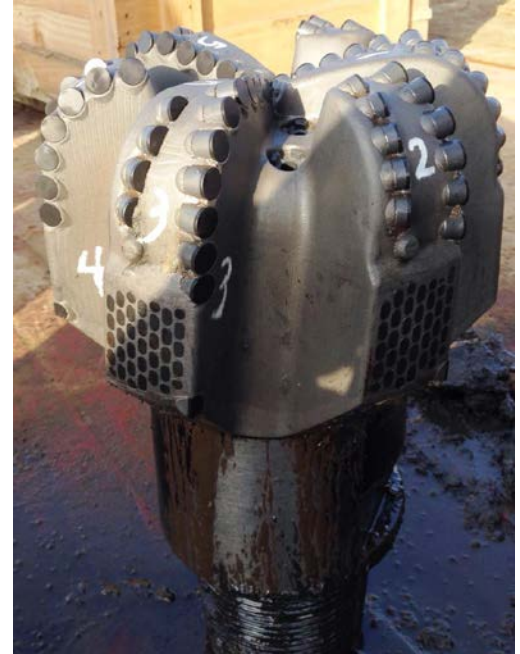
Dull picture provided after drilling two wells without repairs.
