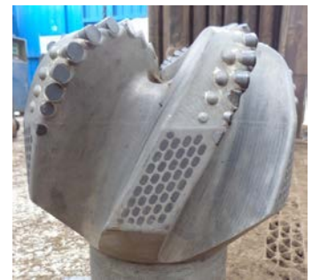
Both bits were pulled with a 1-2 dull grade.
