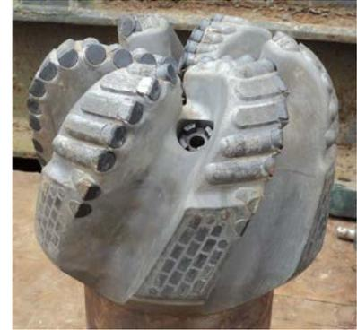
Pulled with a 1-4-WT dull grade, this had an outstanding dull grade compared to offsets.
