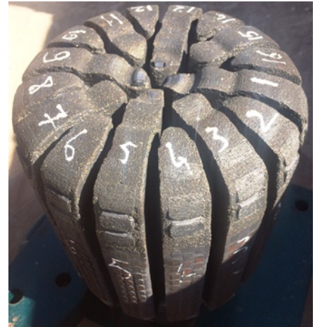
The dull grade after drilling 859 meters was reported as 6-6-WT-A-X-0-NO-CP.
