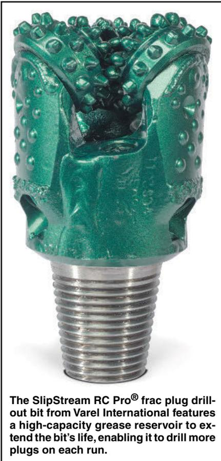
The SlipStream RC Pro<sup>®</sup> frac plug drill-out bit from Varel International features a high-capacity grease reservoir to extend the bit's life, enabling it to drill more plugs on each run.
