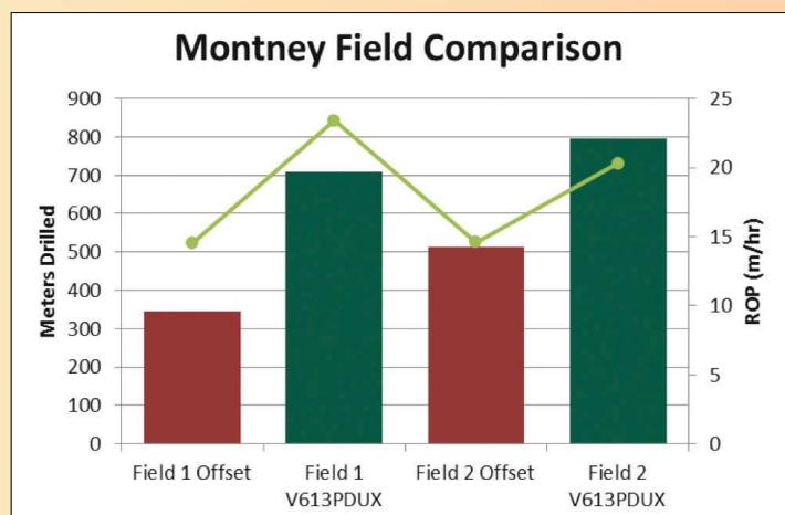
The total number of meters drilled and ROP both increased in the Montney Formation using a new diamond material composition that was incorporated in the cutter. The composition was developed in the Varel Technology Center. (Source: Varel International)
